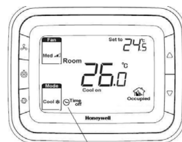
INDICATES THERMOSTAT HAS BEEN SET TIME OFF
